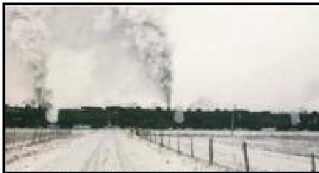
Double headers passing at Monroe siding. Ones throwing smoke are topping grade. Two on right have stopped on siding. No wreck about to happen! Note road crossing sign has no crossbucks. (Wintertime.)
